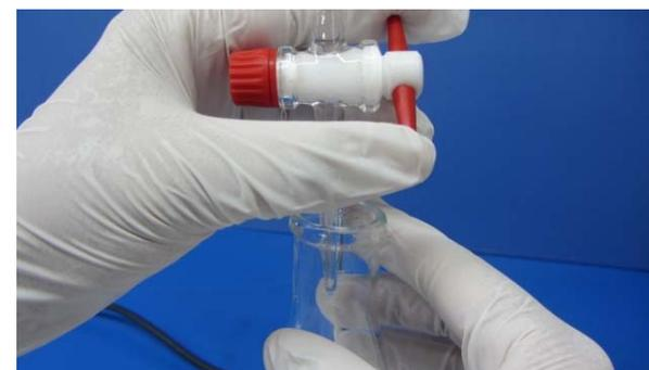
Filter out the ppt. to get saturated  $\text{AgOAc}$  soln quickly to keep the low temp of mixture
